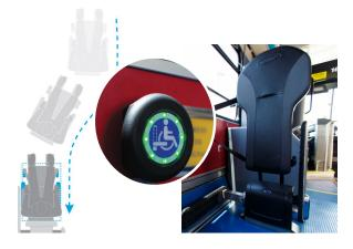
**1.** Back into the space with your wheelchair or scooter, centering it against the backrest, and engage the automatic locking sequence by pressing an ADA-friendly button.
