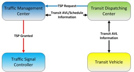
Figure 6: TSP System Architecture – Center-to-Center based
