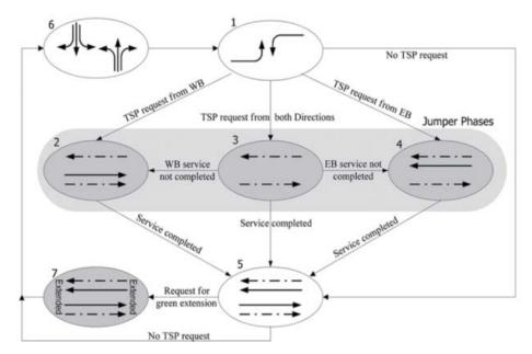
Figure 2: Example of Actuated TSP Phase for Queue Jump
