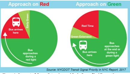
Figure 1 shows the concept of how the green extension and early green/red truncation active TSP logics operate.
