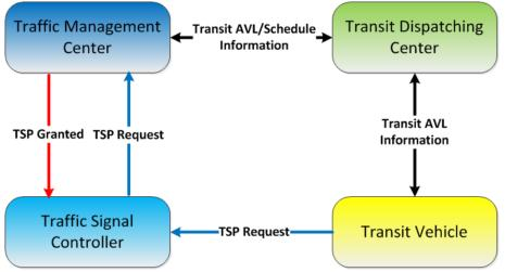
Figure 5: TSP System Architecture – GPS/AVL-based and/or CV-based
