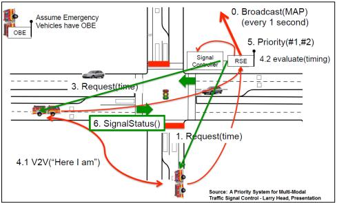
Figure 3: Traffic Signal Priority in the Connected Vehicle Environment
