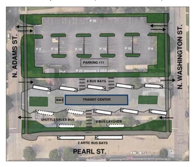
After extensive study and public involvement, a basic functional design has been proposed (above). There are other potential configurations. Many decisions remain. At a minimum the new facility must provide space to accommodate more buses and a larger building. The proposed transit center program yields a 6,500 square-foot building on a 2-acre site and includes the following minimum program elements:
