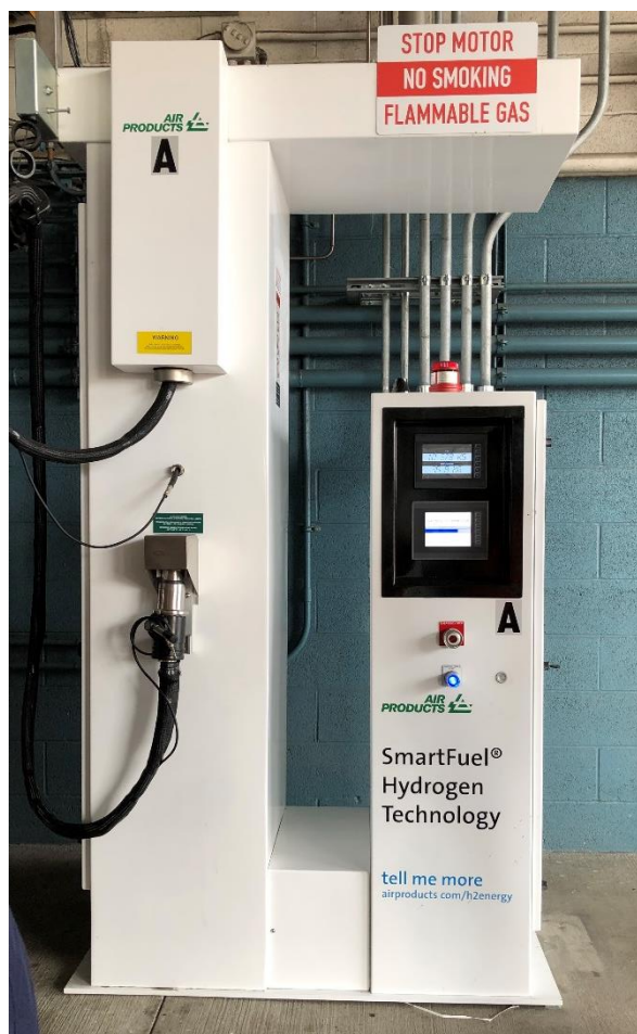
Figure 56: Hydrogen fuelling dispenser, Orange County, California.
